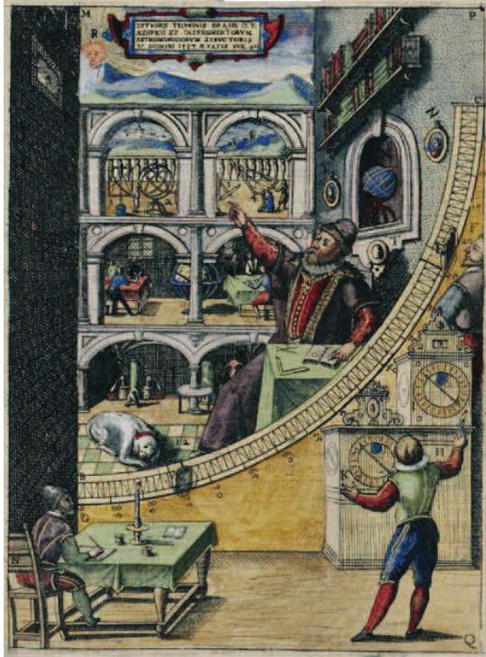
Fig. 2.1. Each graduation of Tycho's quadrant is diagonally divided into ten segments each having six arc minutes, which in turn allows interpolating the measured angle with an accuracy of about one minute.
